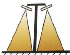
Wall-mounted (Tunnel lighting)
