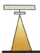
Suspend-mounted (Baylight High / Low)
