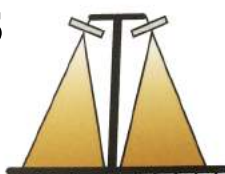
Wall-mounted (Tunnel lighting)
