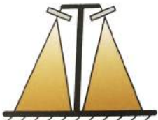
Wall-mounted (Tunnel lighting)
